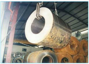
Coils at storehouse with severe rust damage.
